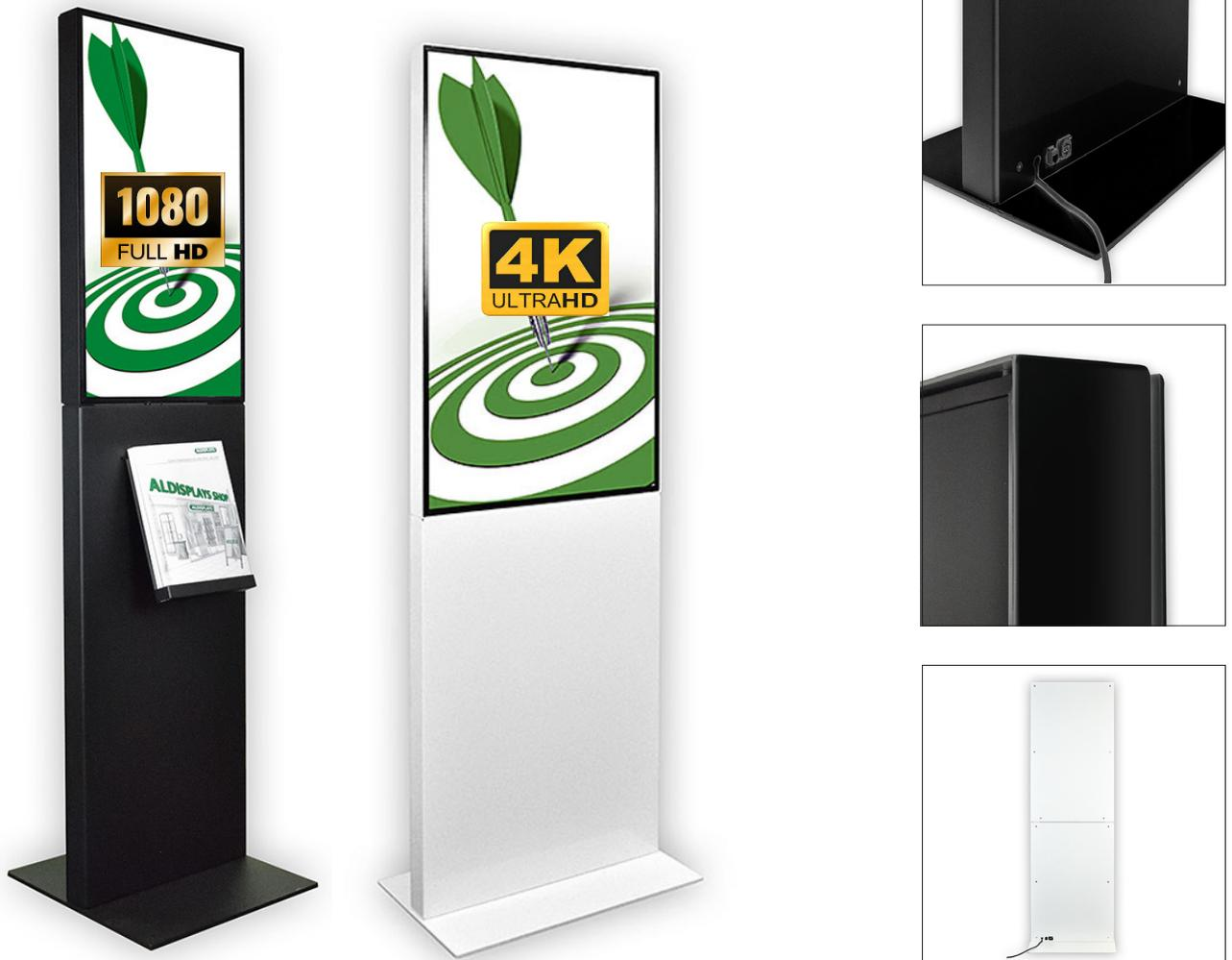
The digital info column TrendLine (66/79mm depth) is made almost frameless of sheet steel and aluminium and is available in 32" and 43" as well as in black and white. (powder-coated according to RAL 9003 and RAL 9005.) The lightweight design eliminates the need for fans and a glass pane on the front surface. The light design allows the still quite simple transport. The 32" stele comes with a removable DIN A4 tray delivered.
