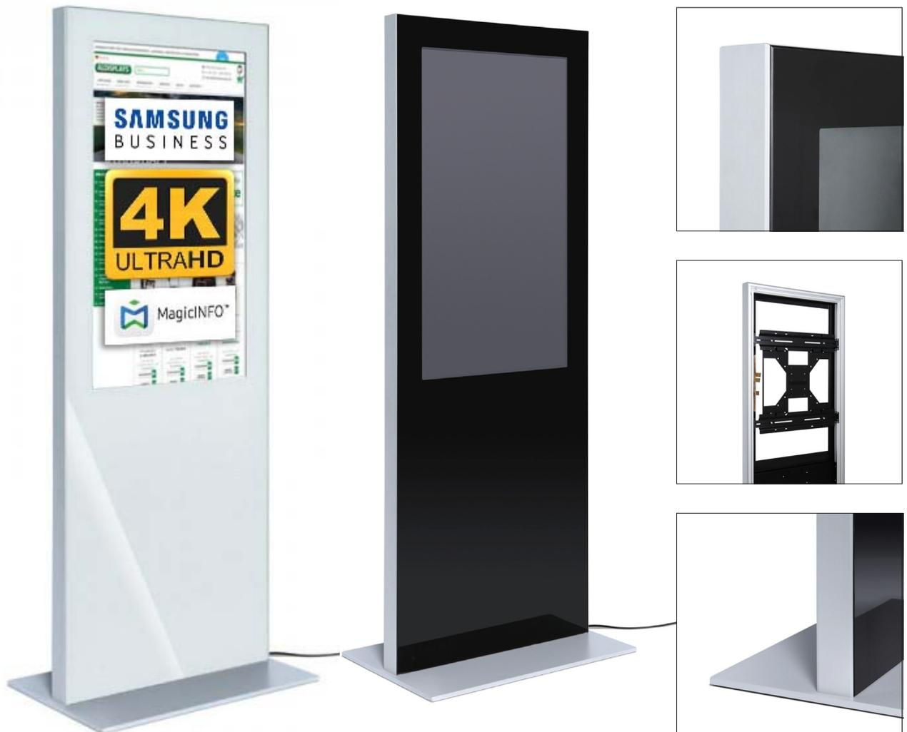
The Digital Info Stand - slim (72mm) made of silver anodised aluminum profile, a heavy steel stand featuring (10 mm, powdercoated according to RAL 9016) as well as a front window made of safety glass. The backside is vaulted with a steel sheet, which is secured with two locks and to operate the professional 24/7 LED displays from Samsung can be opened. Available in black and white.
